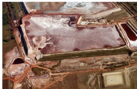
Fig. 10 One year later. Dry mud stacking of press filtered bauxite residue.
