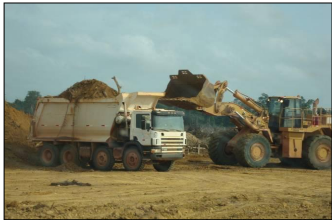
Fig 3 – Detail of the loading of ore by CAT 988H wheel loader
